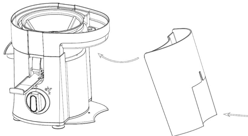
4. Install the top cover onto the top of the juice collect tray as shown in the diagram.
