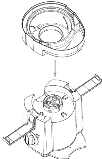
2. Install the filter ASM into the connector at the top of the main body as shown in the diagram.
